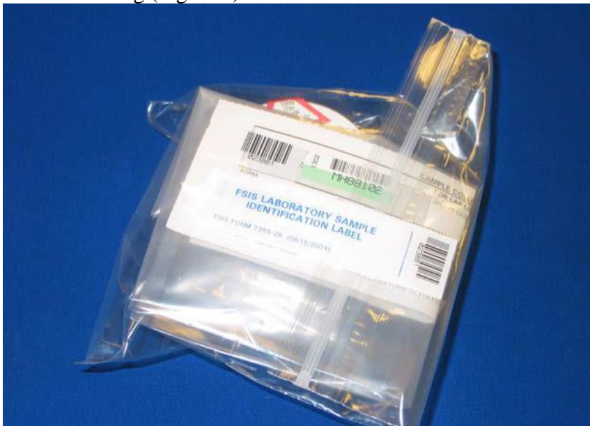
Figure 5 – Assure that the barcode number on the form matches the barcode number on the sample bag
