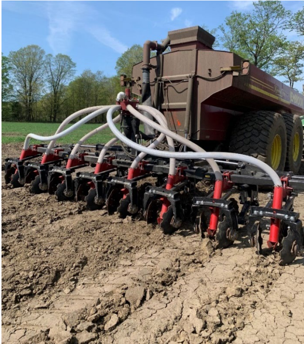
Shanks fracture soil around the injection slot, resulting in moderate disturbance as shown here on cropland.
