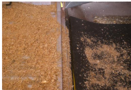
Rubber mat used on ramp at truck exit
