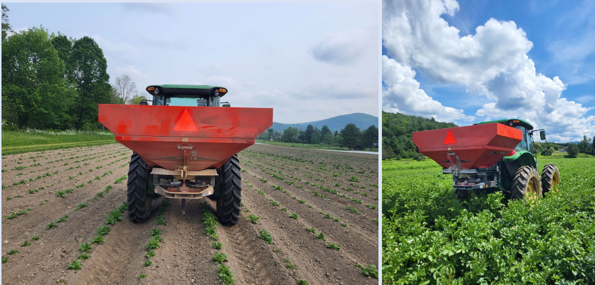
Figure 6. Fertilizer applicator utilized for precise and accurate placement of fertilizer to support crop growth while minimizing overapplication and reducing runoff to nearby waters.
