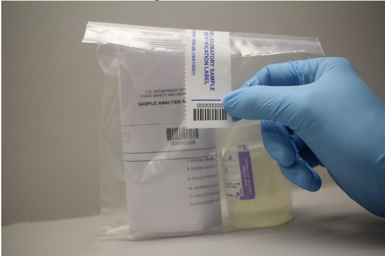
Figure 3. Placement of the identification label on the resealable bag containing the sample and the sample submission form (which is protected in a separate plastic sleeve).
