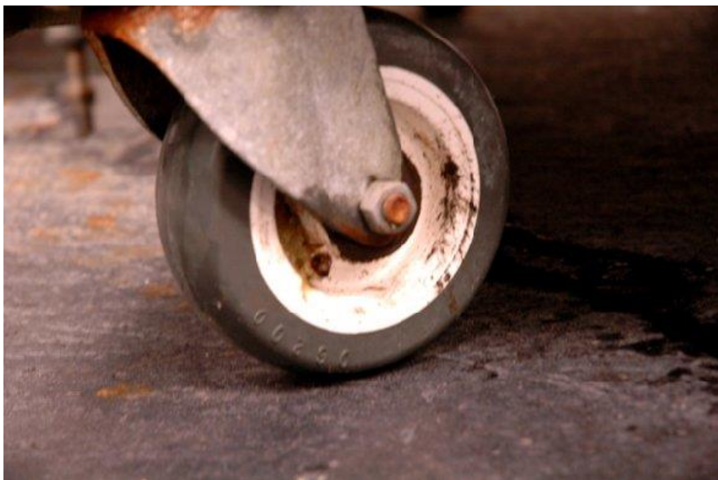
A cart wheel with rust and product residue build up. The wheel can be contaminated with Lm when it is rolled across drains and wet areas in the floor. The Lm can then spread through the establishment when the cart is pushed into different areas.
