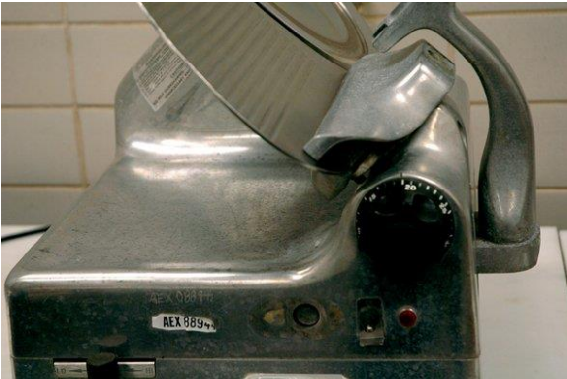
A slicer blade with grime and black residue under the blade. The blade can be contaminated with Lm and spread to the product that is sliced. The slicer handle, controls, and seals may also be contaminated, as these areas may not be frequently cleaned.
