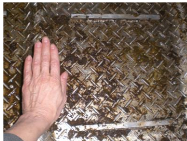
Good footing prevents slips and falls Square stock welded to truck floor Non-slip flooring in new stock trailer
