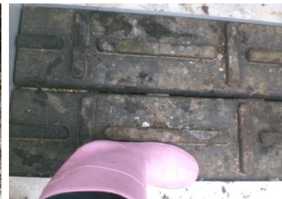
Good footing prevents slips and falls Square stock welded to truck floor Non-slip flooring in new stock trailer
