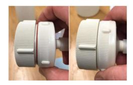
7. Pull the water sample into a Luer tipped 60 ml syringe until the plunger is well-above the 60 mL mark (see below, left). Connect the Luer tip of the syringe to the Luer fitting on the filter apparatus. Push about 5 ml of water through the filter, discarding the filtered water.
