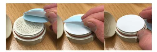
6. Place the filter top on the filter base, twist counter-clockwise until the threads click into alignment, then twist clockwise to screw two pieces together. As the filter top begins to overlap the orange O-ring on the threaded neck of the filter base, you'll feel resistance. Continue to firmly twist until the gap between the filter top and base is closed (see above, right).
