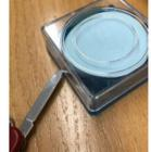
5. Each filter is sandwiched between two discs of light blue paper. Lift out a 'filter sandwich' handling the discs at the edges. Carefully discard the bottom blue disc and position the filter on the filter base (see below).
