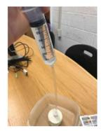
8. Place the sample tube in a rack placed on a stable surface. Place the outlet of the filter apparatus on the uncapped sample tube (below, left) and push water through the apparatus until the water level in the sample tube nears the black 50 ml line. Push lightly on the syringe to slow the flow from a stream to dropwise (below, center). Add dropwise until the meniscus is just touching the top of the 50 ml line (below, right).
